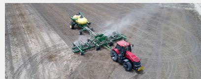
Figure 3: Sowing V071 on top of the ground with an air seeder mimicking dry broadcast.
